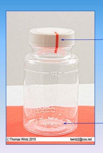
Sterile Seal should remain intact until time of collection (remove after collection & recording of chlorine residual)
