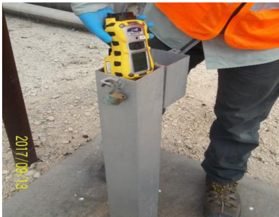
Air monitoring at MW-1 at the start of sampling. Date/Time: 09/13/2017 10:27 a.m.
