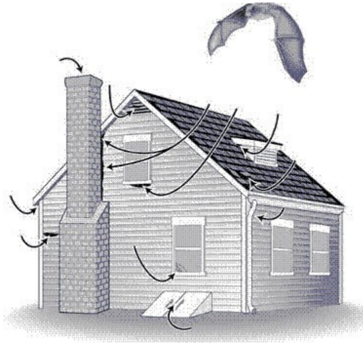
Figure 1: Examples of Openings Where Bats May Enter and Leave Structures.
